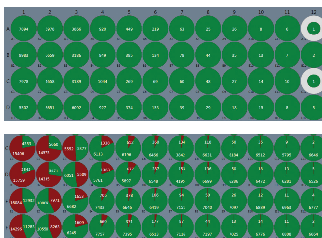
Figure 1: Representation of wells containing multiple fluorescing cells. Top) Single channel output. Bottom) Dual channel output.
