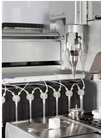
Classic Hopper uses active stirring for uniform flow rate
