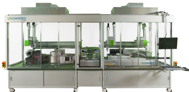
Figure 1: Unchained Labs' freeslate system configured for biologics formulation. The freeslate system on the right prepares formulations and analytical samples, measures pH and viscosity, and performs visual inspection. The freeslate system on the left accesses the Wyatt DynaPro® Plate Reader II Dynamic Light Scattering (DLS) instrument and Molecular Devices SpectraMax® Microplate Reader. A low-bioburden HEPA enclosure encompasses the entire system and work space.
