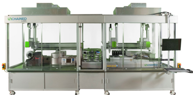
Figure 1: The freeslate system configured for biologics formulation. The robot on the right prepares formulations and measures pH, viscosity and visual inspection. The left robot integrates with the Wyatt DynaPro II dynamic light scattering (DLS) instrument and Molecular Devices SpectraMax microplate reader. A low-bioburden HEPA enclosure encapsulates the system.
