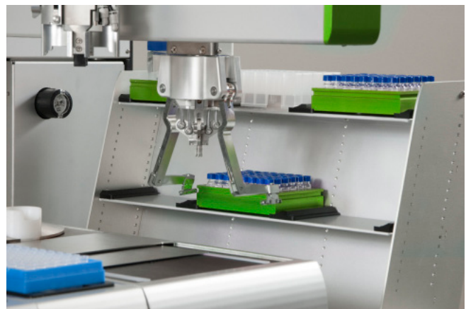
Figure 2: The freeslate jr. for powder dispense taking a plate from the integrated shoulder hotel to the balance.
