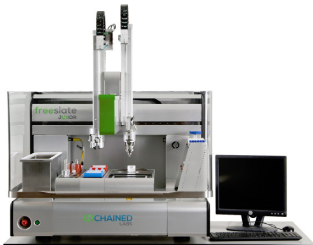
Figure 1: The freeslate jr. for powder dispense.
