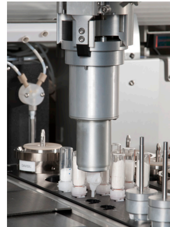
SV dispensers use vibration for precise delivery
