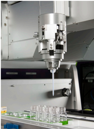
Viscous liquid dispenser handles up to 1000 cP
